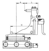
The wheel dresser that dresses two angles tangent to a radius in one continuous motion with .0001 0.002m/m accuracy.
